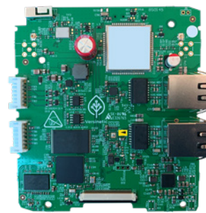
▲ This smart chargepoint communications controller board is an OCPP communications gateway for smart chargers connecting ISO 61851 controllers to back-offices via Ethernet, Wi-Fi or LTE Cellular networks.
