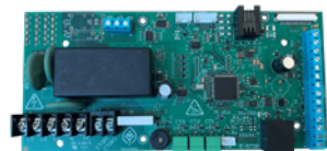
▲ This AC charge controller, for single- or three-phase EV chargers, interfaces with control boards such as the one pictured above to support smart charging.
