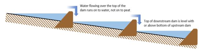
**Figure 3.4 | Optimal spacing of dams.** Dams should be installed using a 'top-to-toe 'principle to avoid undercutting and erosion. On average, dams should be placed every 7-12m, depending on slope, and water should fill the entire section between dams. Pictures adapted from Moors for the Future Partnership fact sheets.
