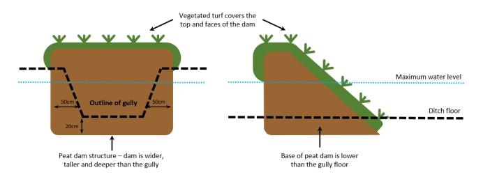
Figure 3.1 | The construction of a peat dam. Showing the front view (left) and the side view (right) of peat dam construction. The vertical edge of the dam is on the downstream side of the dam. Pictures adapted from Moors for the Future Partnership fact sheets.
