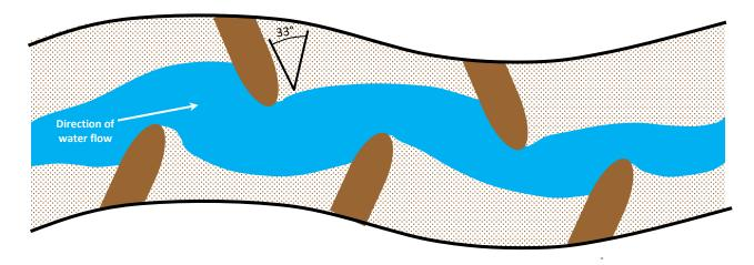
Figure 3.6 | Baffle placements down a large gully. Optimum placement will be to avoid bank erosion, thus keeping the main water flow in the centre of the gully and away from the re-profiled edges.
