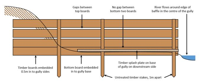
Figure 3.8 | A timber baffle. An example of a timber baffle. Diagram adapted from Moors for the Future.
