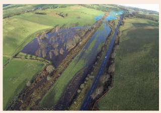
Figure A1.8 Eddleston Water re-meandering (stage 1) in flood conditions (courtesy Tweed Forum)
