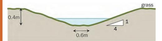
Figure A5.1 Cross-section through proposed swale
