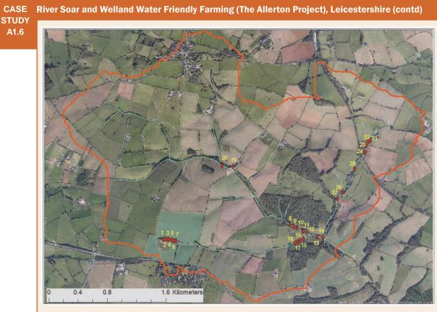
Figure A1.20 Leaky barriers in the Eye Brook catchment. Installation dates and total capacity are: barriers 1 to 7, September 2016, 887 m<sup>3</sup>; barriers 8 to 18, September 2017, 8090 m<sup>3</sup>; and barriers 19 to 27, September 2018, 8697 m<sup>3</sup> (courtesy Water Friendly Farming)
