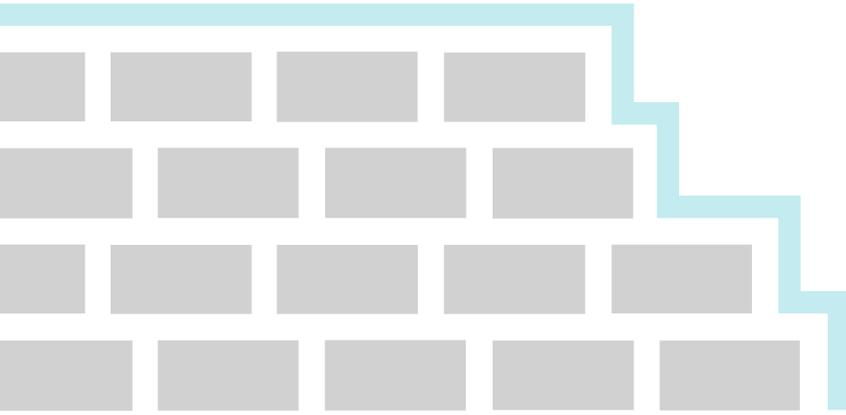
External wall insulation involves fitting layers of insulation and an external protective layer, usually rendered, to the outside of the property. External pipework, guttering, windowsills and other fitting may need to be moved or extended, and scaffolding is usually required.
